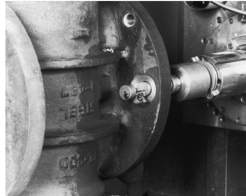
Back spotfacing large valve body.
