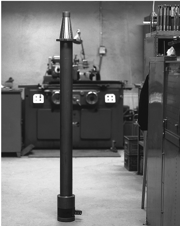
Special tool to operate in a diesel engine block.
